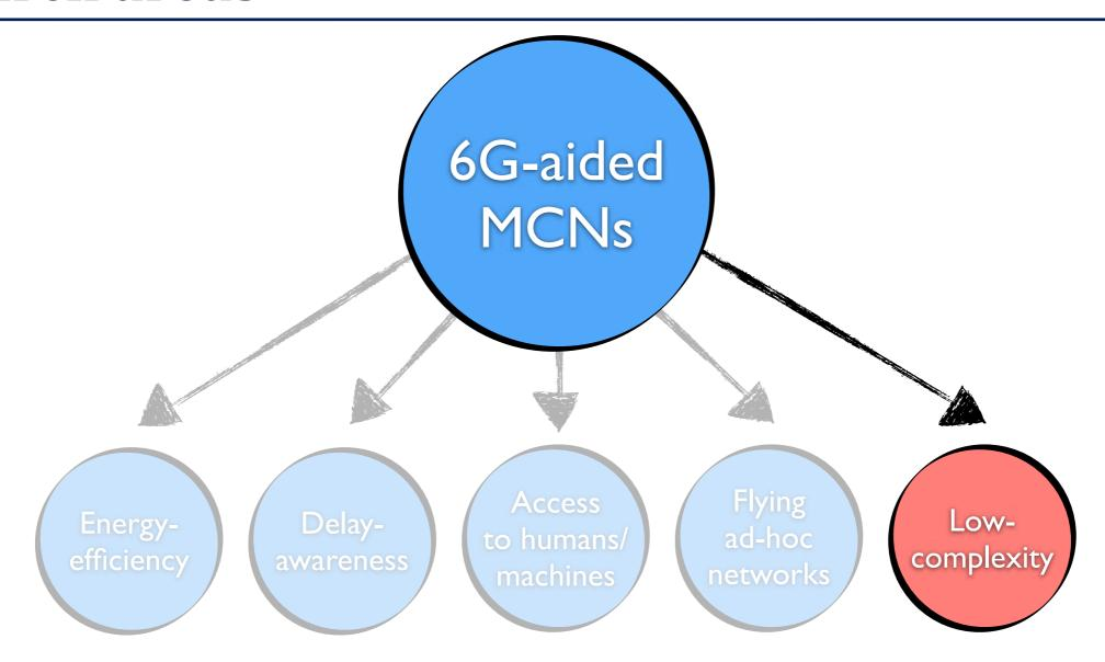
Avoid excessive network coordination overheads to support the massive number of users and IoT devices
